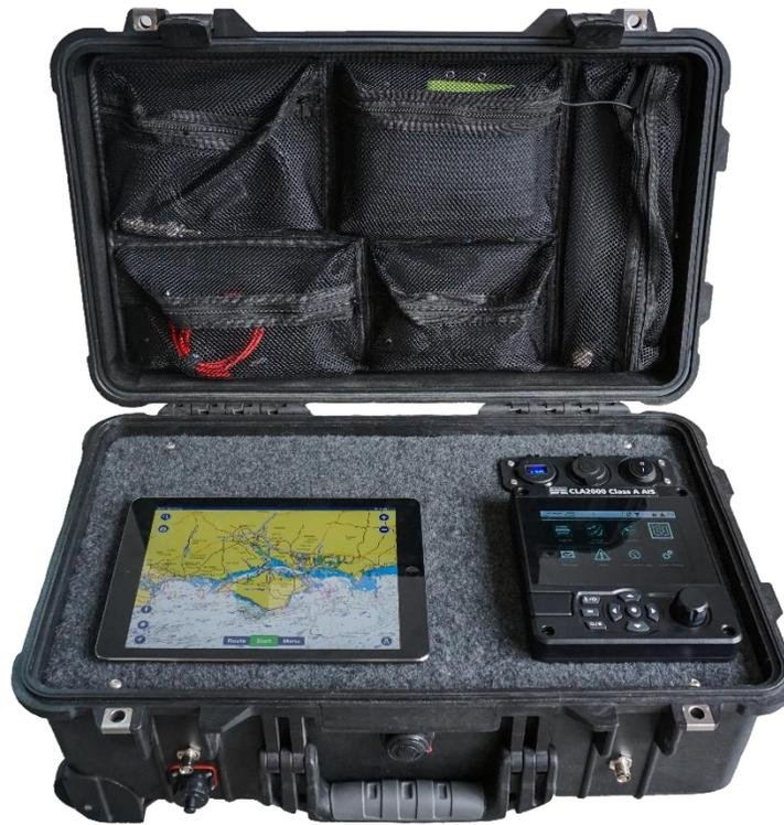
AIS Deploy is autonomous with integrated, rechargeable 12v 22Ah battery and portable GPS and VHF antennas. It's also designed for transportation using a standard aircraft cabin friendly format, ultra rugged, waterproof Pelicase
