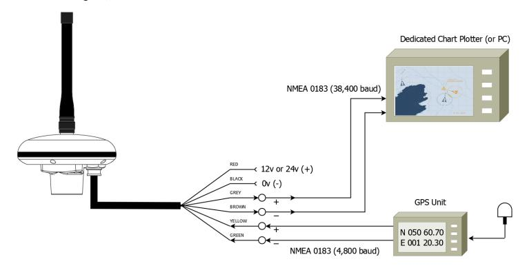
NOTE: Connection of the GPS Unit to the ANT200 is not mandatory but can be useful in some installations where the dedicated chart plotter only has one NMEA Input port
