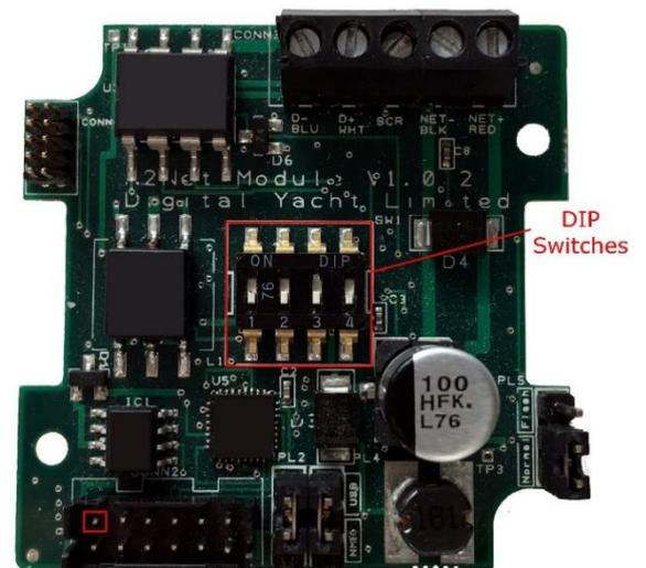
Once you have set the DIP switches, power cycle the veKonvert unit for the new Device Instance to be applied.
