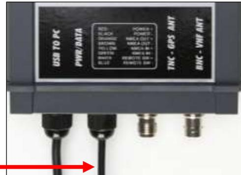
The most common connection to a dedicated chart plotter is to take the NMEA Output (Orange+ and Brown –) from the CLB1000 Transponder and to connect it to a free NMEA Input on the plotter. You must then tell the chart plotter that AIS data is connected to this port and set the baud rate to 38,400 Baud – the standard speed for AIS data. Consult the instruction manual supplied with your Chart Plotter to understand how this is configured.
