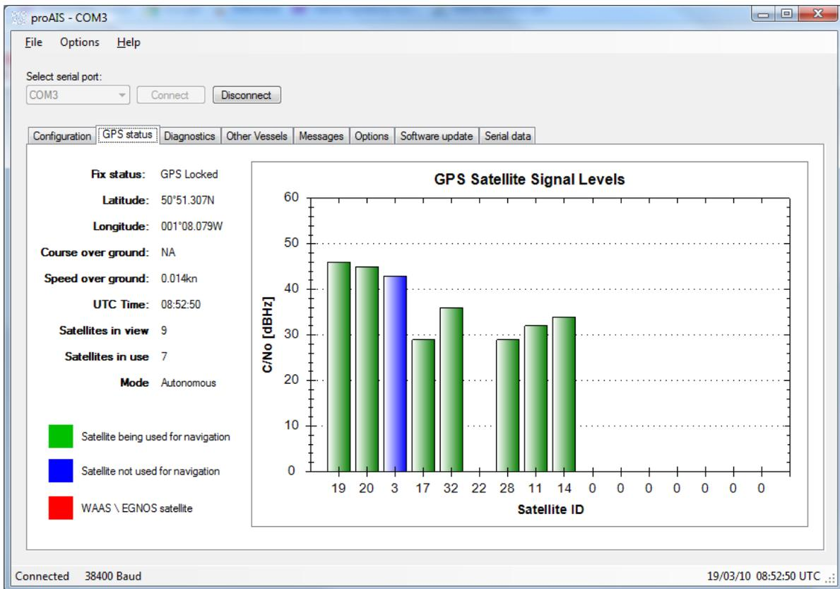
Satellite signal strength bars are shown in green for satellites that are currently being used for navigation. Blue signal strength bars are used to show satellites not currently being used for navigation. It is normal for the graph to display a combination of green and blue bars.
