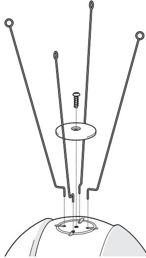
Figure 5 Attaching the bird deterrent
