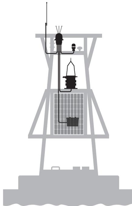
Figure 2 Typical AIS AtoN system
