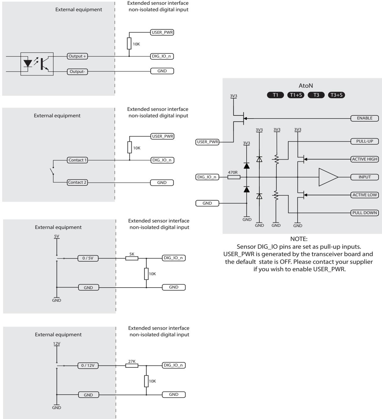
Figure 17 Non Isolated digital input reference circuit
