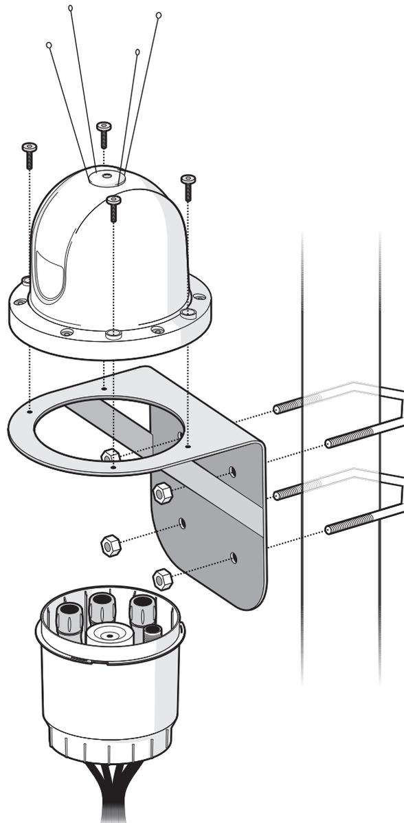
Figure 6 Using the mounting bracket
