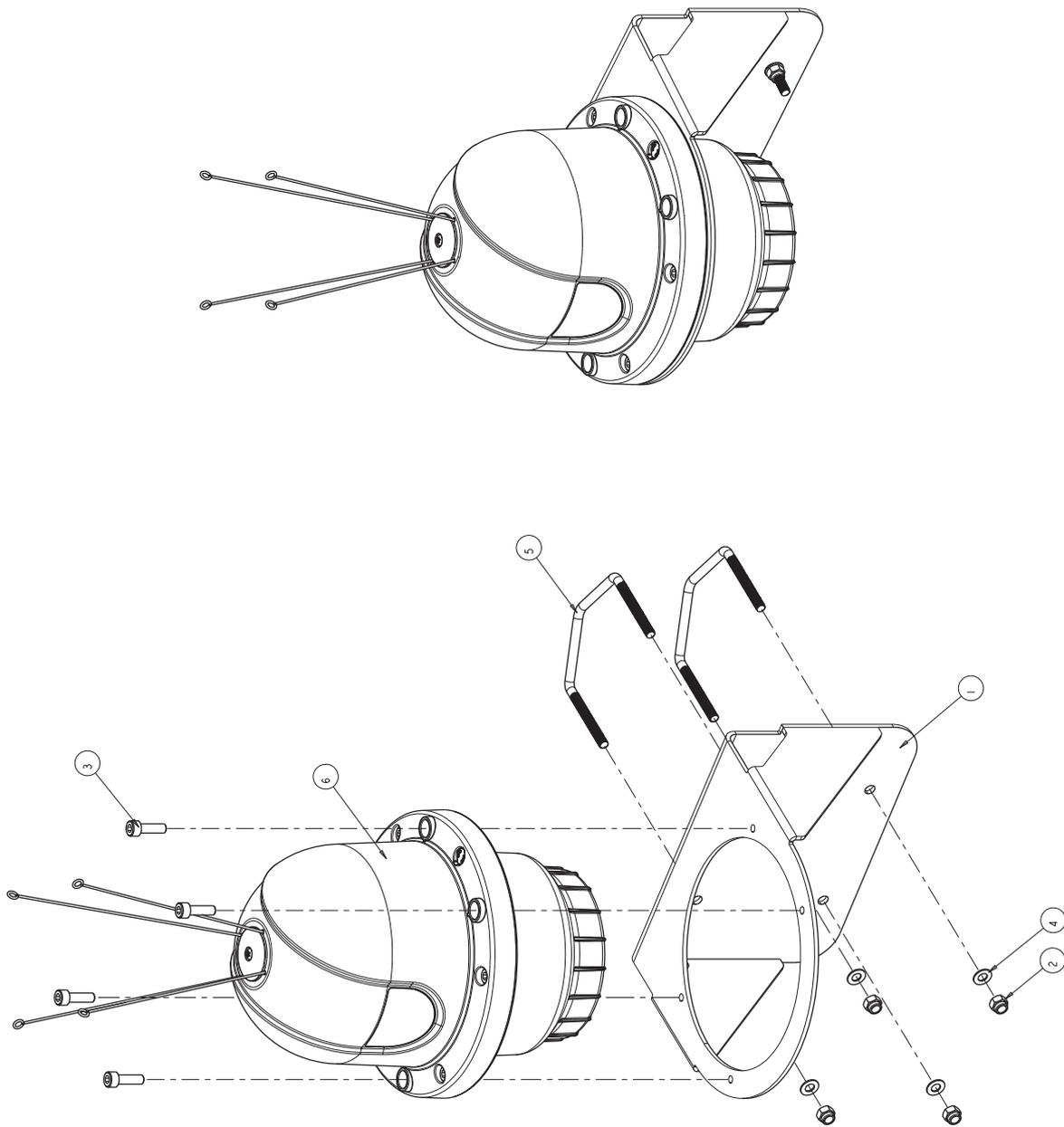
Figure 35 Transceiver general assembly
