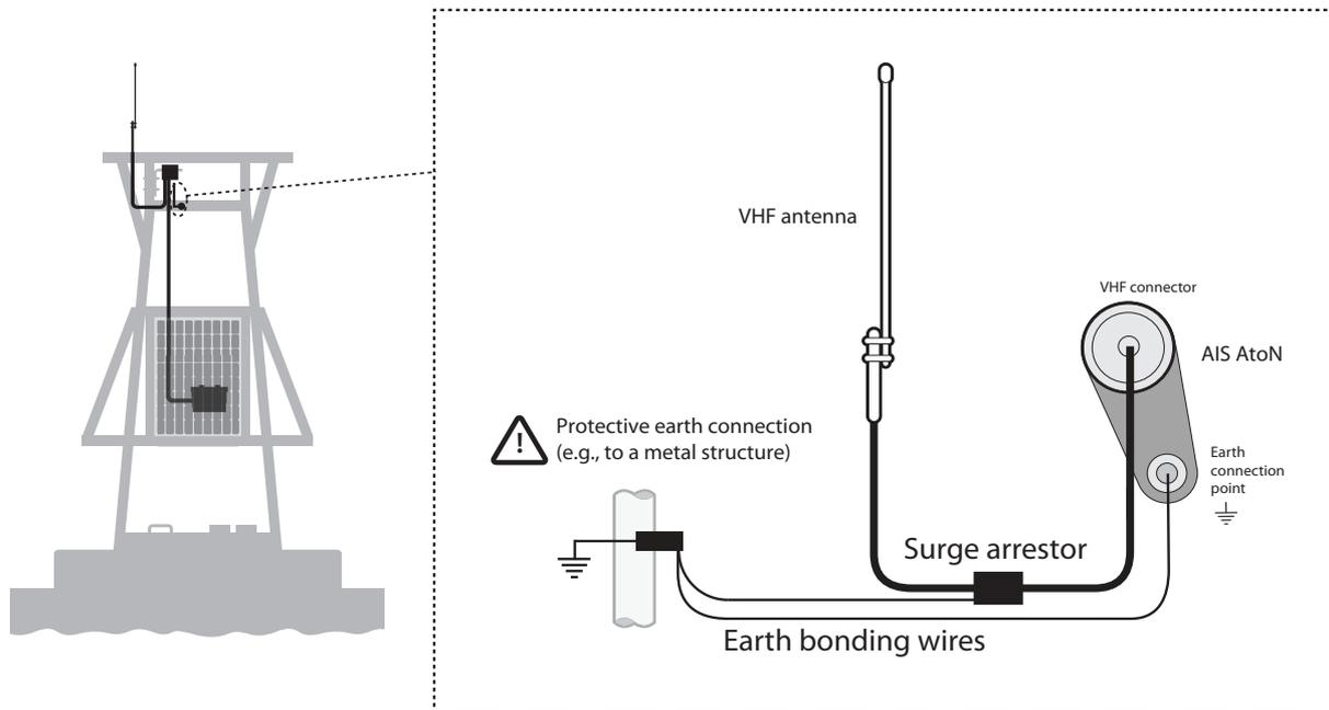
Figure 12 VHF antenna connection
