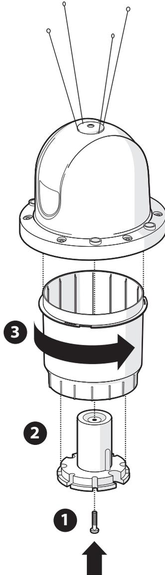
Figure 8 Removing the connector cover
