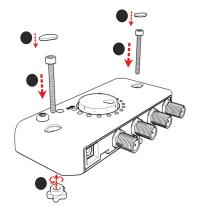
The amplifier should be mounted in a dry location close to the TV. It is not waterproof. In general, permanent access is not required as it will only be necessary to occasionally adjust the antenna gain or to twitch the amplifier on/off
