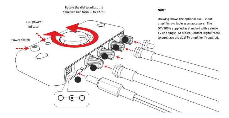
Run the RG6 coax cable assembly and connect to the ANT INPUT connector
