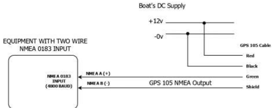
When connecting to a single wire NMEA Input (such as Garmin), connect the GPS105 Green wire to the NMEA + Input and the Screen/Shield to the Power – (0v).
