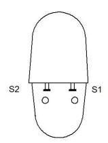
When the HSC100 is viewed from the front face, Switch 1 is on the right and Switch 2 is on the left.
