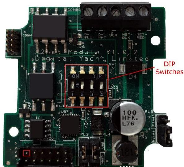
By default iKonvert is set to Mode 0, where all of the four DIP switches are OFF. In this mode it will convert all of the common GPS/Nav/Instrument data at 4800 baud.
