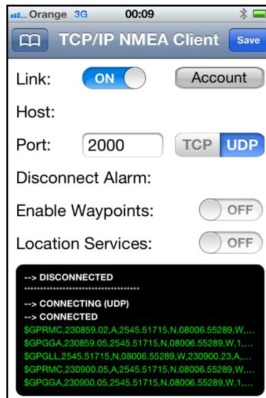
This proves that the iNavHub is correctly converting NMEA 0183 data to wireless data which can be used in any UDP compatible app that you wish to use.
