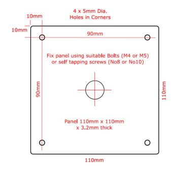
Secure the switch plate using suitable bolts of self tapping screws (not supplied).
