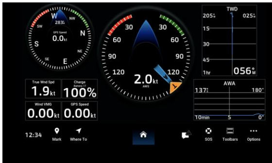
Figure 4 State of charge of the Calypso Unit and wind data on a Garmin GPSMAP
