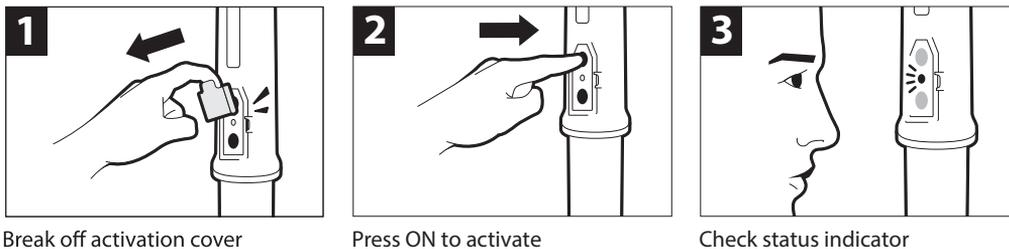
Figure 6 Activation procedure
