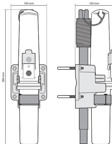
Figure 5 AIS SART overall dimensions
