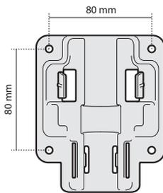
Figure 4 Dimensions for bracket mounting holes
