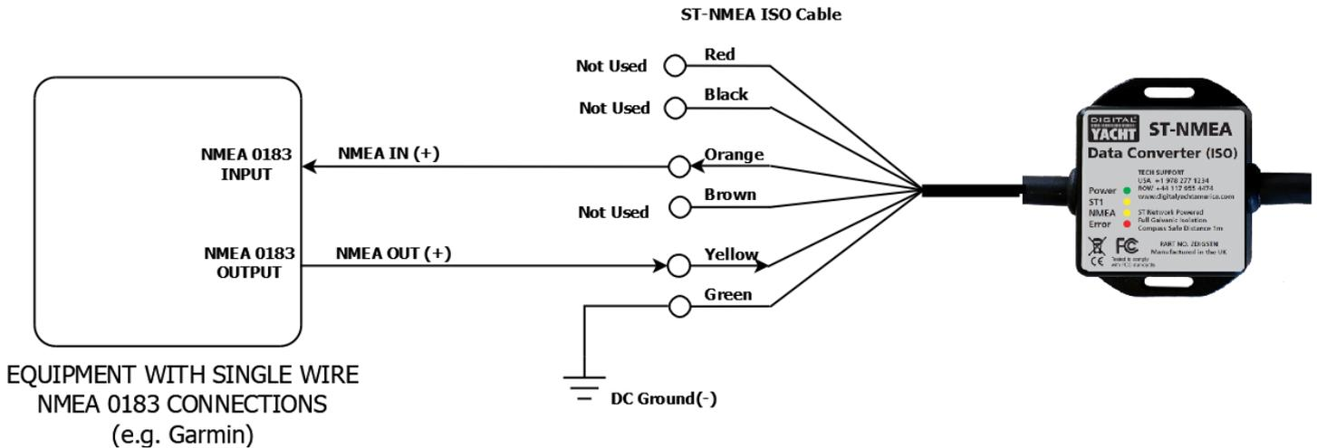
Below is a typical connection diagram for connecting the ST-NMEA Converter to a 2 wire NMEA0183 Devices, which are now what you will find in the majority of new systems and are fully NMEA0183 compliant.
