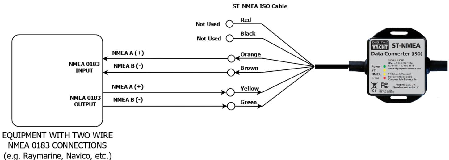
The Red and Black wires in the ST-NMEA ISO cable are not power connections, but a single Input and Output wire which we have reserved for future use.
