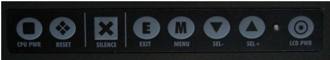
Press the “Menu” key to enter the OSD Mode. Use the “Up” and “Down” Arrow keys to select the menu you need and then press the “Menu” key to enter that menu. Every menu has an option “Exit” which when selected returns you to the previous menu or if in the main menu exits the OSD Mode.
