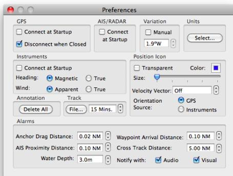
In most situations, it is also worth ticking the “Connect at Startup” tick box and this will make MacENC automatically connect to the GPS and AIS data, each time you run MacENC.
