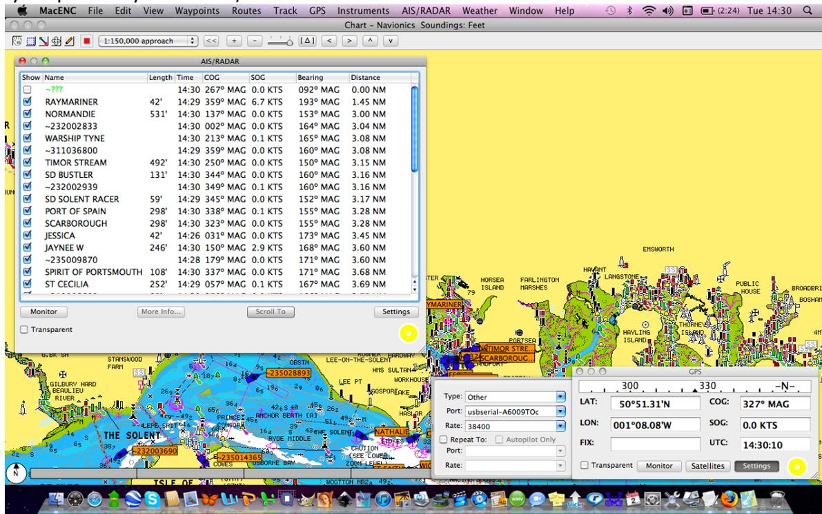
To display a list of the AIS targets that are currently being displayed, from the menu bar click "AIS/RADAR" and then select "Connect". The AIS/RADAR window will then be displayed (shown above). You can sort this list in various ways and also select individual targets to display more information about them or scroll to them on the chart (centres the chart on the selected AIS target).
