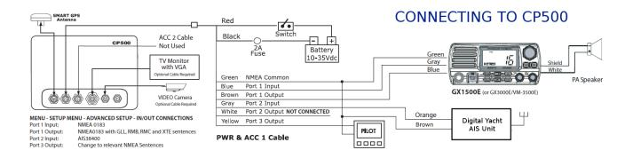
The following diagrams are applicable to the Digital Yacht ANT200 Smart AIS antenna.
