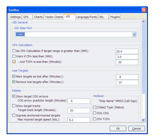
For Windows the drop down selection list will list COM ports and in this example we have selected COM15. To find out what COM port your AIS has been allocated by Windows you may have to run the Device Manager application and look in the "Ports (COM&LPT)" section. Refer to <u>Tech Note 00001-2010</u> for more info on this.
