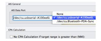
For LINUX the drop down selection list will look like this and you want to select the "/dev/ttyUSB0" device or similarly named device, not the "/dev/ttysX" devices which are conventional serial ports.
