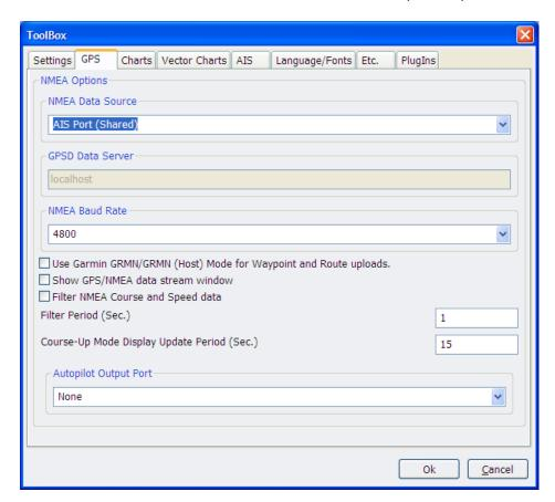
If you just have an AIS receiver and want to use an existing separate GPS connection then don't change the NMEA Data Source setting and keep the existing settings that you had before, assuming that the GPS position was already working correctly.
