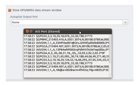
The "\$GPxxx,xxx,.....\*nn" type messages are from the GPS and the !AIVDM,xxxx......\*nn" type messages are from the AIS.
