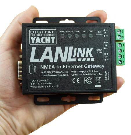
LANLink is available in two versions suitable for NMEA 0183 and NMEA 2000 respectively. It features an easy to use web interface allowing any device with a browser to configure NMEA baud rates and IP/Port information.
