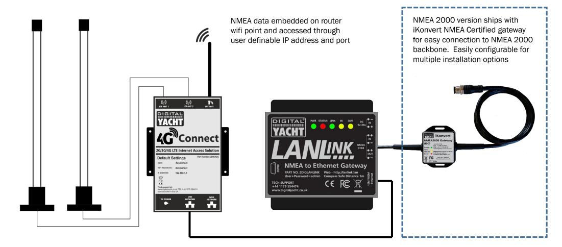
Simple ethernet patch cable connection to router
