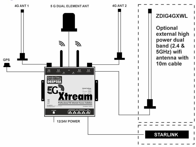
5G Xtream features independent dual band (2.4 & 5GHz) wifi for interconnection to mobile devices.
